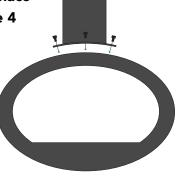
On recessed ceilings with plasterboard or similar plates, the fireplace should prefarably be attached to one of the overhead joists behind the ceiling plates to ensure that the ceiling can support the weight of the fireplace.
