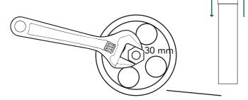
Turn to the left to loosen the tube and determine the height of the fireplace.
